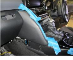
TIP: Take a 400mm piece of 50mm paper masking tape and fold 100mm at end back on itself. Stick the remainder to the trim. This can then be used as a handle to allow better leverage to pull the trim backward.
